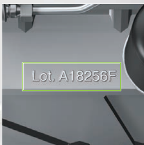
Presence inspection of marked characters
